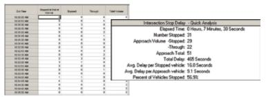
Signalized Intersection Delay studies are based on standard methods used by traffic engineers and provide a statistical method for measuring delays. Reports provide total volume recorded during the study, broken down into vehicles that were delayed at the signal, and those that went though without delay.
