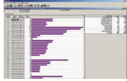
The overall data is analyzed for Average Stopped Time, Maximum Stopped Time, Average Queue, and Queue Density, among other statistics. This type of study can also be done for an approach to a signalized intersection.
