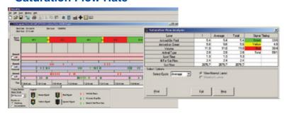
PETRAPro allows you to quickly and easily produce reports for saturation flow rates at intersections. These rates are based on actual real-time data, and not on predefined values that may or may not be accurate. Depending on how the data has been collected in the field, PETRAPro can process and analyze the data for not only Saturation Flow rate, but also vehicle headways, lost times, arrival types, signal timings & approach volumes.
