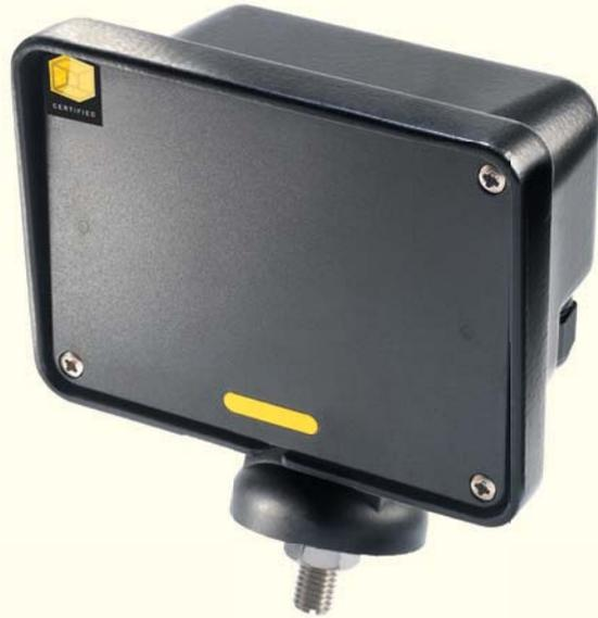
This product has been designed to be mounted externally on vehicle actuated signs (VAS). It provides the main detection function at remote sites where solar power supply is typical. The 335 FMCW radar operates in the 24GHz band.
